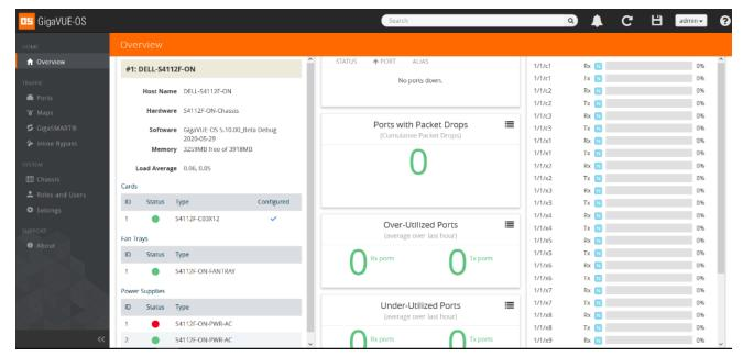
b. Select **Chassis** from the left navigation pane and choose 'List View' to view the details of the chassis, line card, hardware, and environment.
